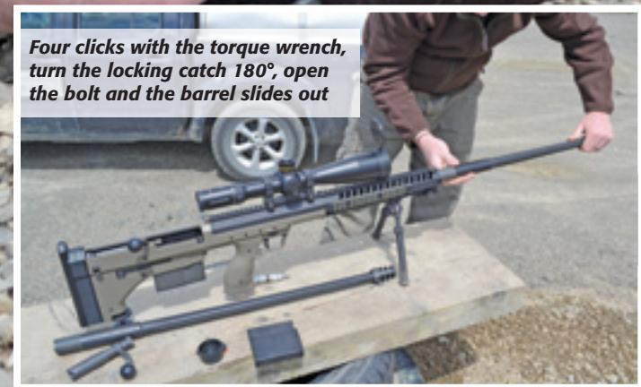
*Four clicks with the torque wrench, turn the locking catch 180°, open the bolt and the barrel slides out*
